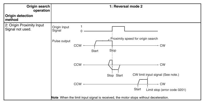
Specifying the Origin Search Direction (CW or CCW Direction) Sets the direction to move when detecting the Origin Input Signal.
