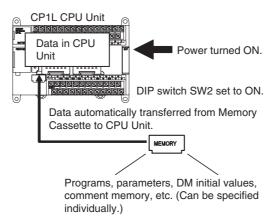
This function can be used to copy data to another CPU Unit without using the CX-Programmer.
