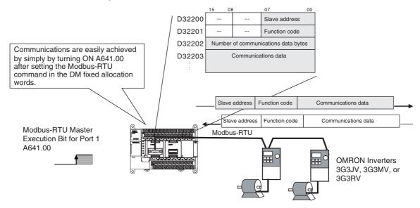
DM Fixed Allocation Words for the Modbus-RTU Easy Master
