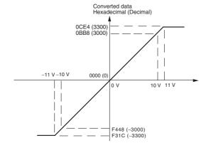
Voltage in the -10 to 10 V range corresponds to hexadecimal values F448 to 0BB8 (-3,000 to 3,000). The range of data that can be converted is F31C to 0CE4 hex (-3,300 to 3,300). A negative voltage is expressed as two's complement.
