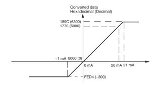
Current in the 0 to 20 mA range corresponds to hexadecimal values 0000 to 1770 (0 to 6,000). The range of data that can be converted is FED4 to 189C hex (-300 to 6,300). A negative current is expressed as two's complement.
