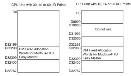
This data area is used for general data storage and manipulation and is accessible only by word.
