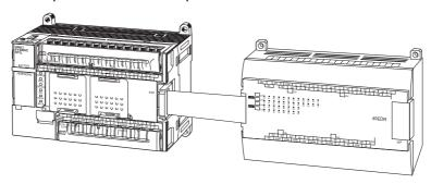
3. Replace the cover on the CPU Unit's or the Expansion I/O Unit's expansion connector.
