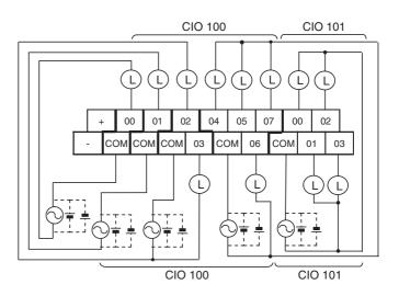
AC-power-supply models have a 24-VDC output terminals (+/-) on the lower terminal block. They can be used as a DC power supply for the input circuit.
