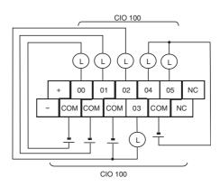
AC-power-supply models have a 24-VDC output terminals (+/-) on the lower terminal block. They can be used as a DC power supply for the input circuit.
