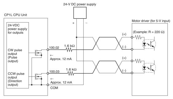
In this example, a 5-V input motor driver is used with a 24-VDC power supply. Be careful to ensure that the Position Control Unit output current does not damage the input circuit at the motor driver and yet is sufficient to turn it ON.
