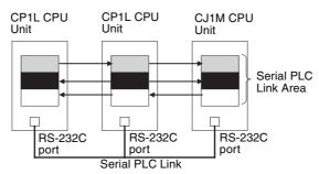
Addresses not used for Serial PLC Links can be used in programming, the same as the Work Area.
