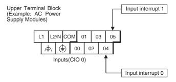
Input Terminal Block of CPU Units with 14 I/O Points
