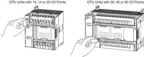
2. Holding the Memory Cassette with the side with the nameplate facing upwards, insert the Memory Cassette all the way into the slot.
