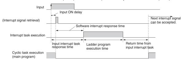
The time from completing the ladder program in the input interrupt task until returning to cyclic task execution is  $60~\mu s$ .
