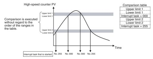
**Note** The range comparison table can be used without starting an interrupt task when the comparison condition is met. The range comparison function can be useful when you just want to know whether or not the high-speed counter PV is within a particular range.
