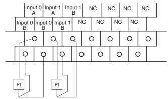
Temperature input 0 Temperature input 1
