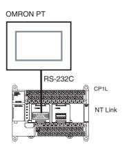
With the NT Link protocol, the PLC automatically responds to commands sent from the PT, so no communications programming is required in the CP1L.
