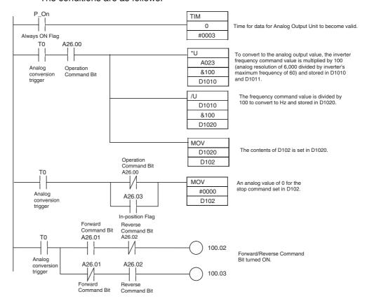
In this example, the results of \*U and /UL are 1, so the value in A23 is moved directly to D102 with MOV.
