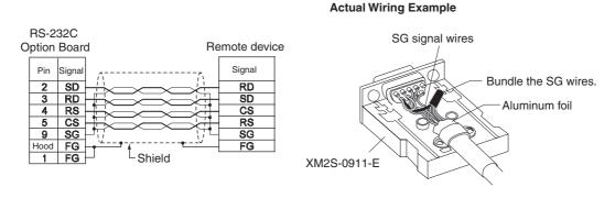
**Note** The Hood (FG) is internally connected to the ground terminal (GR) on the CPU Unit. Therefore, FG is grounded by grounding the ground terminal (GR) on the power supply terminal block. Although there is conductivity between the Hood (FG) and pin 1 (FG), connect the Hood (FG) to the shield because the Hood (FG) has smaller contact resistance with the shield than pin 1 (FG), and thus provides better noise resistance.
