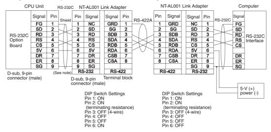
**Note** We recommend using the following NT-AL001 Link Adapter Connecting Cables to connect to NT-AL001 Link Adapters.
