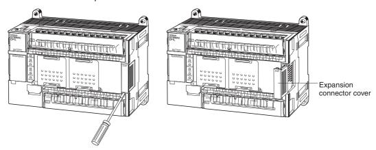
2. Insert the Expansion I/O Unit's connecting cable into the CPU Unit's or the Expansion I/O Unit's expansion connector.
