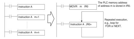
If, for example, instruction A above is a comparison instruction, table data could be read from start to the end of the table to compare all of the data with a specific value. In this way, blocks of user-defined processing can be freely created depending by applying Index Registers.
