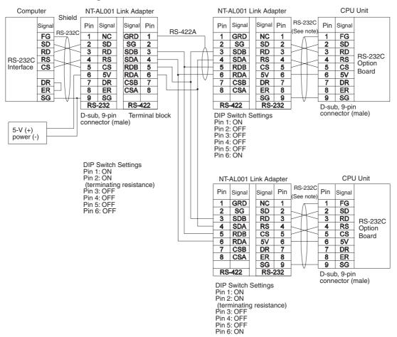
**Note** We recommend using the following NT-AL001 Link Adapter Connecting Cables to connect to NT-AL001 Link Adapters.
