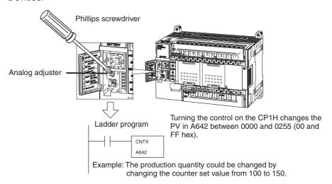
Changing Settings Using External Analog Setting Inputs
