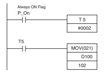
TIM 005 will start as soon as power turns ON. After 0.1 to 0.2 s (100 to 200 ms), the Completion Flag for TIM 005 will turn ON, and the data stored in DM 0100 will be moved to IR 102 as the conversion data for analog output 1.
