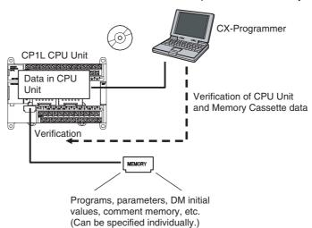
This function can be used for operations such as confirmation after data has been written to the Memory Cassette, or confirming that the data in the backup matches the data in the CPU Unit.
