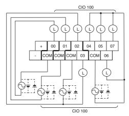
AC-power-supply models have a 24-VDC output terminals (+/-) on the lower terminal block. They can be used as a DC power supply for the input circuit.
