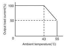
(3) CP1W-32ER's maximum number of simultaneously ON output points is 24 (75%). Design the system considering the simultaneously ON points and load current based on the following curve.
