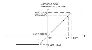
Voltage in the 0 to 5 V range corresponds to hexadecimal values 0000 to 1770 (0 to 6,000). The range of data that can be converted is FED4 to 189C hex (-300 to 6,300). A negative voltage is expressed as two's complement.
