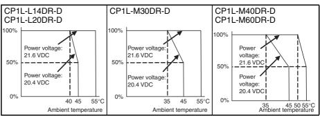
**Note** The above restrictions, apply to the relay output load current from the CPU Unit even if Expansion I/O Units are not connected.
