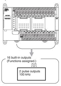
**Note** The instruction used to control each output point determines whether it is used as a normal output, pulse output, or PWM output.
