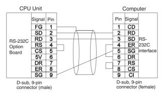
Using NT-AL001 Converting Link Adapters
