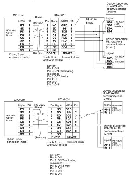
**Note** We recommend using the following NT-AL001 Link Adapter Connecting Cables to connect to NT-AL001 Link Adapters.
