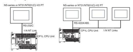
Note Communications are not possible using the 1:1-mode NT Link protocol.
