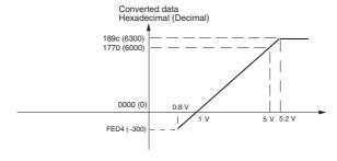
Voltage in the 1 to 5 V range corresponds to hexadecimal values 0000 to 1770 (0 to 6,000). The range of data that can be converted is FED4 to 189C hex (-300 to 6,300). Voltage in the range of 0.8 to 1 V is expressed as two's complement.
