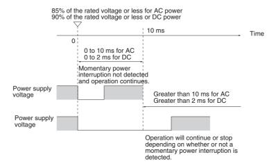
The following timing chart shows the CPU Unit power OFF operation in more detail.
