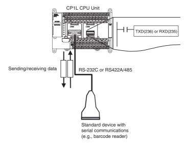
For example, simple (non-protocol) communications can be used to input data from a barcode reader or output data to a printer.
