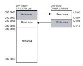
CP1L is set as the link master, so CIO 3000 to CIO 3007 are its write area. Any data written to these words with the OUT or MOV instructions will be automatically transferred to LR 00 to LR 07 in the CPM2A. The CPM2A will use these words as its read area.
