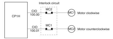
This circuit prevents outputs MC1 and MC2 from both being ON at the same time even if both PLC outputs CIO 100.00 and CIO 100.01 are both ON, so the motor is protected even if the PLC is programmed improperly or malfunctions.
