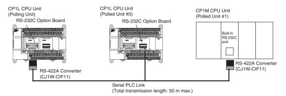
**Note** The CP1W-CIF11 is not insulated, so the total transmission distance for the whole transmission path is 50 m max. If the total transmission distance is greater than 50 m, use the RS-422A/485 port on the CP1W-CIF12 directly, or the insulated NT-AL001, and do not use the CP1W-CIF11. If the CP1W-CIF12 or NT-AL001 is used, the total transmission distance for the whole transmission path is 500 m max.
