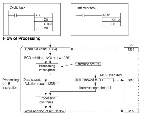
The interrupt occurs during processing of the +B instruction and the result is saved temporarily without being written to the destination word (D0).
