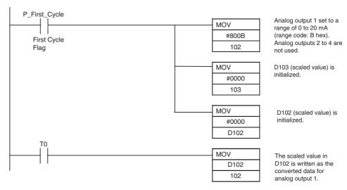
Refer to the first line in the programming example in *Referencing the Automatically Calculated Inverter Frequency Command Value* on page 334 for a timer for the time required for the Analog Output Unit's data to be valid (analog conversion trigger: T0).
