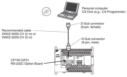
Connect the CX-Programmer to the RS-232C port of the CP1W-CIF01 Option Board by XW2Z-200S-CV/500S-CV RS-232C cable.
