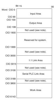
**Note** The parts of the CIO Area that are labelled "not used" may be used in programming as work bits. In the future, however, unused CIO Area bits may be used when expanding functions. Always use Work Area bits first.
