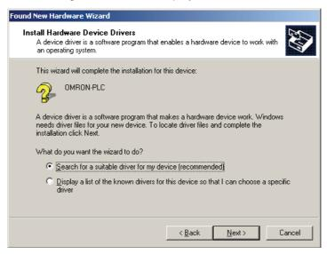
Select the Search for a suitable driver for the device (recommended) Option and then click the Next Button. The following window will be displayed. From the list in the window, select the Specify location Checkbox and then click the Next Button.
