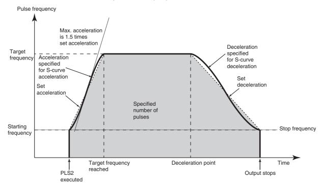
The same type of S-curve acceleration/deceleration can be used for ACC(888) as well.
