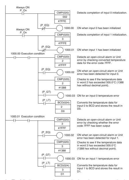
The following programming example shows how to convert the data for temperature input 0 to BCD and store the result in D0 and D1. "0001" is stored in D1 when the input data is a negative value. The following system configuration is used.
