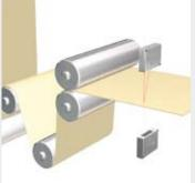
The thickness of permanent lines such as pasta dough or biscuit is a vital factor in the production process. Pastry that is too thin or thick will result in quality problems and raw material wastage. Random sampling and inspection does not offer reliable results, as defective goods are often detected too late. By applying two optoNCDT140SC sensors, the thickness can be measured easily and continuously. The signals are directly used for controlling the production line.
