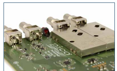
PicoScope 2206 front-end screening
