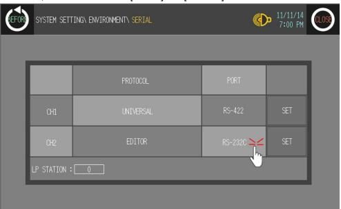
To check baud rate, data bit, stop bit, parity, etc, touch 'SET'.
