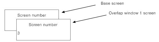
Overlap window 2 is not overlapped because the value of overlap window 2 device is not an existing base screen number.
