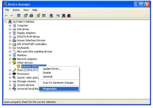
3rd 'Autonics GP/LP Series Properties' dialog box appears. Click 'Reinstall Driver'.
