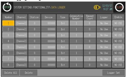
Touch to-be set number as data logger and touch 'Logger Set' and 'PERIOD LOGGING' screen is displayed.
