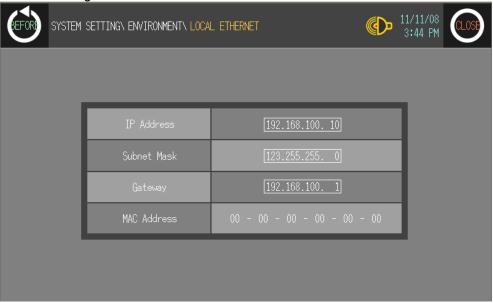
You can designate IP address, subnet mask, and gate way of GP-S070 and check MAC address.
