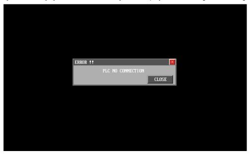
Touch 'CLOSE' and error message dialog box disappears. If connection error is not resolved after 5 seconds, error message appears again on the screen.
