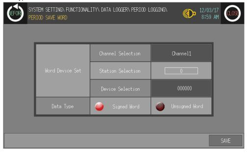
8th Touch 'Device Selection' and input key pad appears to set appropriate device. Enter 'UW' 6.
