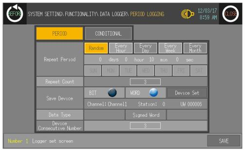
13th Set 'USE' of Enable and data logger function operates.
