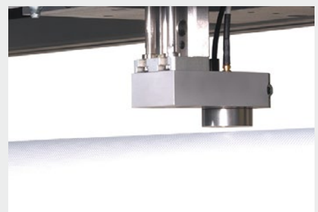
Non-contact, inline thickness measurement of plastic films
