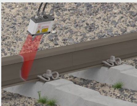
Measuring the inside of the rail
