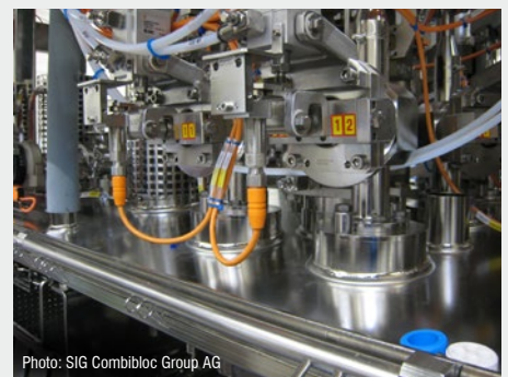
Valve lift measurement in the food industry
