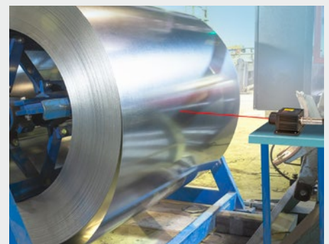
Acquisition of coil diameters
