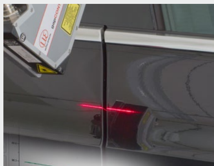
Gap and flushness measurement on bodywork parts
