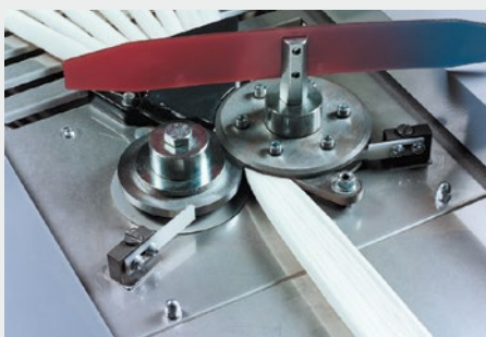
Inline yarn thickness measurement
