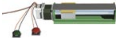
A slider system with a pre-programmed C type Cool Muscle.
